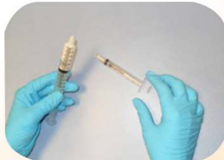
5. The mixture is transferred from one syringe to the other, several times, in order to obtain an homogeneous mixture
