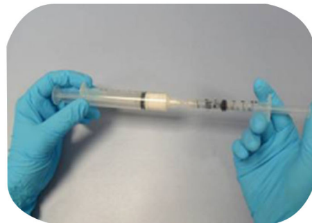
4. The liquid is transferred into the syringe with the powder in order to mix the two components
